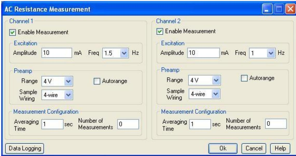
Figure 5-6. The sequence command window for resistance measurements.
