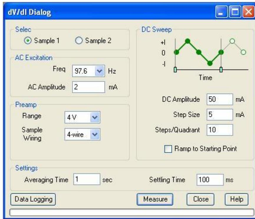
Figure 5-4. The immediate mode differential resistance measurement window.
