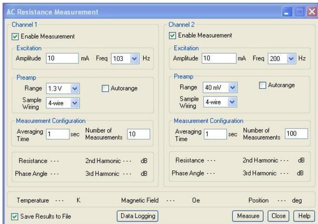
Figure 5-2. The immediate mode AC Resistance Measurement Window.
